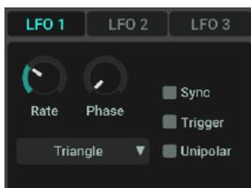
The LFO section offers three independent LFO's per voice with five different waveforms (Triangle, Saw, Rectangle, Random and Noise).
