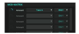
The MOD-MATRIX, allows it to modulate almost every parameter of TAL-SAMPLER. It's also possible to modulate the intensity of another MOD-MATRIX entry. You can have up to 10 modulations.
