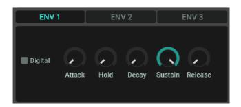
The envelope section provides one ENV1 (AMP) envelope, a ENV2 (VCF filter) envelope and a modulation envelope.
