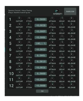
Click on the SC button at the top to open the service control dialog. It allows it to calibrate or detune parameters like cutoff, fine tune and envelope speed for each synth voice and adds analog behaviour to the digital sample engine.
