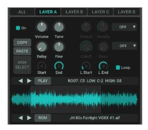
The Layer View shows the individual layer parameters. You will find settings like Volume, Tune (+- 24 halftones), Fine Tune (+- 1 halftone) and delay, where you can delay the sample start up to one second.
