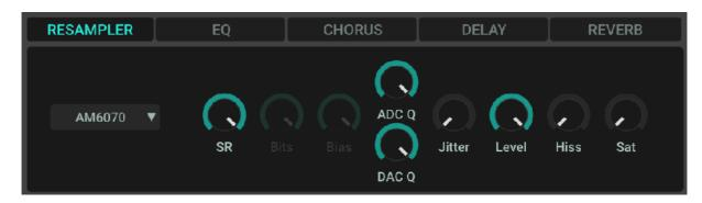
The re-sampler section allows it to change the way samples are re-sampled. There are five modes (DAC types) with a different sound, CPU usage and quality. Every sample that plays will be processed separately.
