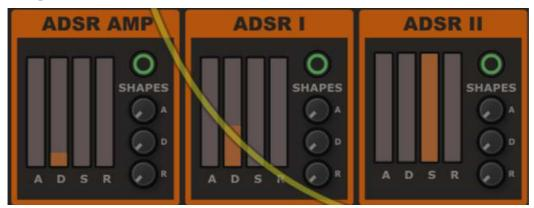
All three ADSR envelopes contain a shape knob for the attack, decay and release part of the envelope. They turn the envelope curve from concave to convex or the opposite. Turn the shape knobs to the middle for linear ADSR's.
