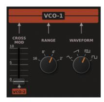
**CROSS MOD:** Controls the cross modulation amount using the VCO-2 wavefom as the source.
