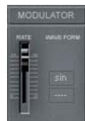
The special thing here is the noise waveform which allows the modulation of PW, filter frequency and VCO frequency with noise.
